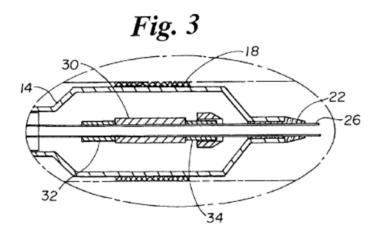
Figure 3 depicts an enlarged cross-sectional view of the distal end of catheter 12, with balloon 14 and stent 18 in expanded states. *Id.* at 2:27–30. As shown in Figure 3, "mounting body 30 . . . is included inside balloon 14 to provide a cushion and/or substrate of enlarged diameter relative to the stent shaft to support and hold the stent and secure it during crimping and
