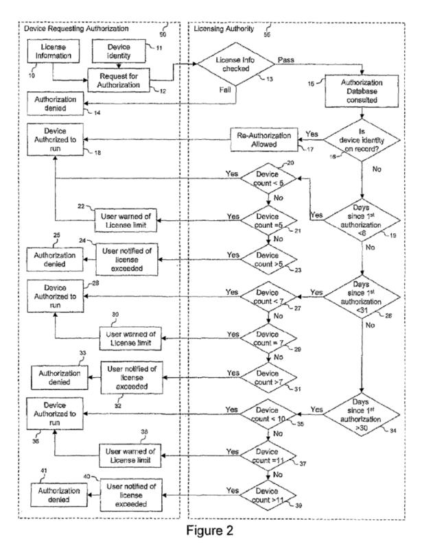
Figure 2 is a flowchart for an approach to adjusting a license for a digital product. *Id.* at 3:20–21. In Figure 2, device 50 requests authorization from
