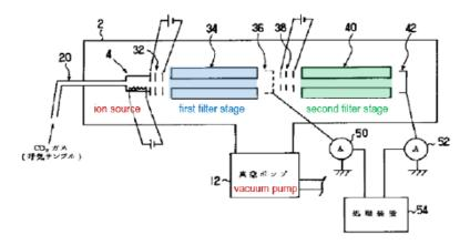
As illustrated in Figure 7, reproduced above, ionizing device 4 emits ions into front stage filter 34, which, in turn, passes certain ions based on its filter characteristics to back stage filter 40. Ex. 1010 ¶¶ 58, 61–65.
