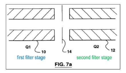
As illustrated in Figure 7a of Douglas, reproduced above, two quadrupoles Q1 and Q2 operate in tandem and in a manner in which both quadrupoles mass select the same ion. *Id.* at 9:13–17, 9:41–46. Although Douglas discloses that each quadrupole may operate at the same constant resolution, Douglas also contemplates that the two quadrupoles may operate at different resolutions. *Id.* at 13:15–16, 13:25–27.
